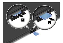
5. To install a SIM card, insert the SIM card firmly into the slot until you hear a click.
